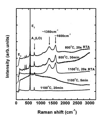
FIG. 4. Raman spectra of C-implanted GaN samples thermally treated at 800 and 1100  $^{\circ}$ C by a RTA with time of 20 s or a furnace annealing for 5, 20, or 30 min.
