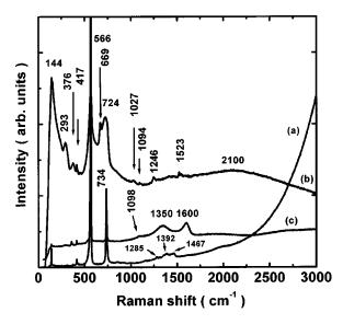
FIG. 1. Raman spectra of: (a) an as-grown GaN sample, (b) a C-implanted GaN sample without annealing, and (c) a C-implanted GaN sample with postimplantation furnace annealing at 800  $^{\circ}$ C for 30 min.
