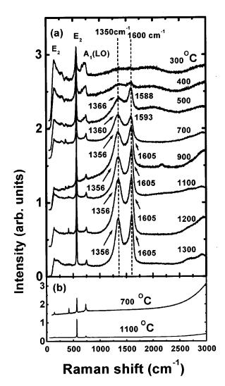
FIG. 2. Raman spectra of: (a) C-implanted GaN samples subjected to RTA with temperatures between 300 and 1300 °C and of (b) two control samples subjected to RTA at 700 and 1100 °C. The RTA time is 20 s for both (a) and (b). The intensities of all spectra are normalized with the  $E_2$  (high) peak intensities taken as a constant.
