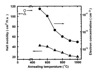
FIG. 5. Electron concentrations and Hall mobilities of a GaN sample before C-implantation (shown by an open circle and an open triangle, respectively), and after postimplantation furnace annealing at temperatures in the range of 500-1000 °C for 20 min (shown by full circles and full triangles, respectively).
