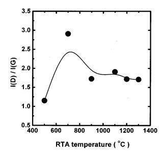
FIG. 3. Ratio of the integrated intensity of the  $\sim$ 1350 cm<sup>-1</sup> band to that of the  $\sim$ 1600 cm<sup>-1</sup> band as a function of RTA temperature.
